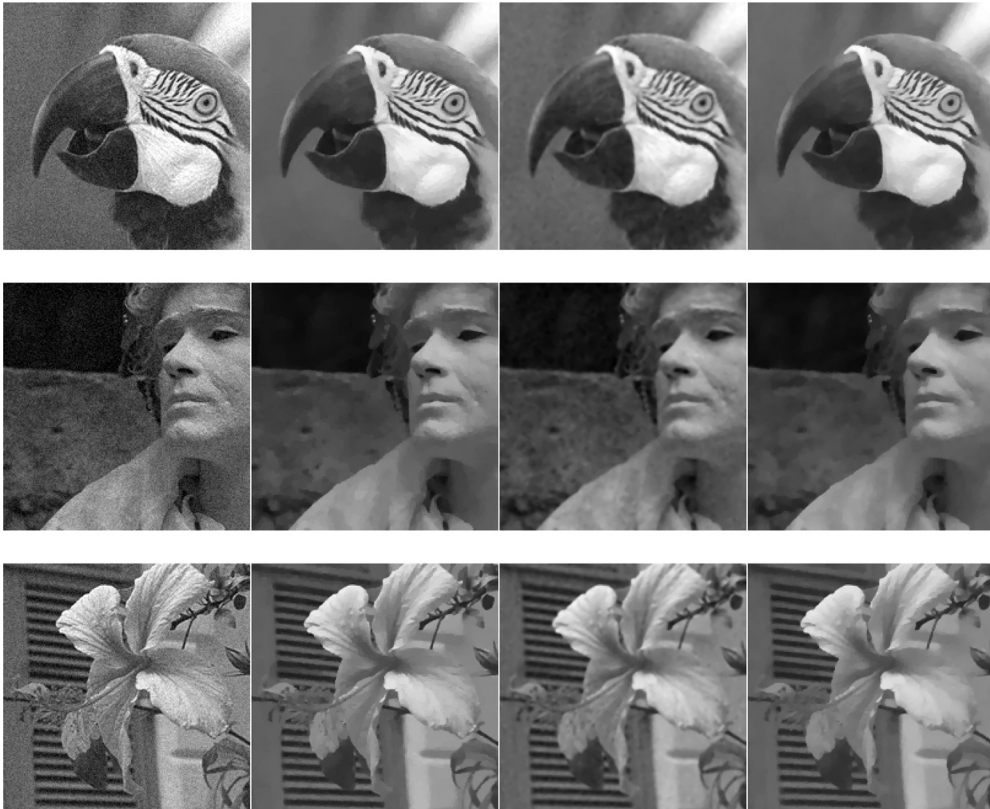
FIG. 6. The noisy images in the first column have additive Gaussian noise with \sigma = 15 . The results from GC model are presented in the second column. They show edge and contrast preservation as well as a fair removal of noise. The results from the MC model, in the third column, tend to have slightly smoothed edges while the background looks not as smooth as expected. The results from the TV model have the well-known problem of blocky regions.
