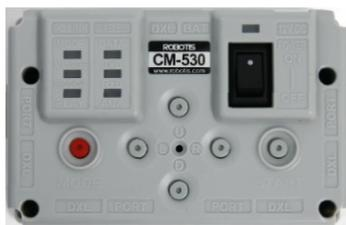
Figura 3 Control CM-530 del robot Bioloid Premium.
